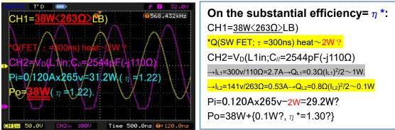
In this 50% up of <u>38W</u> measurement, the efficiency (1.22) seems becoming weaker than  $26W(1.27)_{1}$
