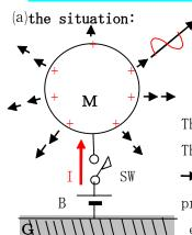
G is earth of voltage=0. B is battery connecting to monopole anttena M through switch SW. M is a sphere of conducting surface. Making SW on causes M equivoltage of B by flowing charge(current) on M.
