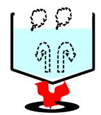
Boiling kettle with convection flow. and hot water evaporation by heating enrgy.
